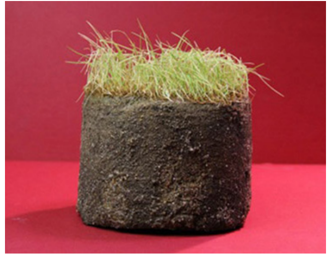
Figure 3. A turf plug with the proper dimensions: approximately 6 inches in diameter and 4-6 inches deep.
