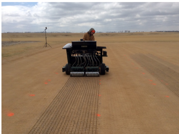
Figure 3. Use a seeder to get good seed to soil contact and cut through dead tissue.
