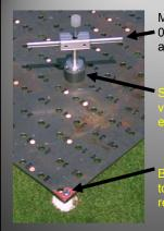
Modified soil probe simulates 0.5" diameter hollow-tine core aeration
