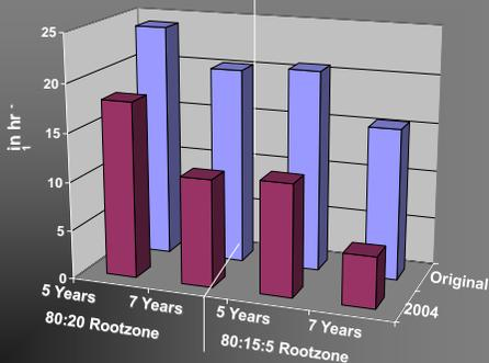
Comparison of preconstruction  $K_{sat}$  values to  $K_{sat}$  values taken 10/04.
