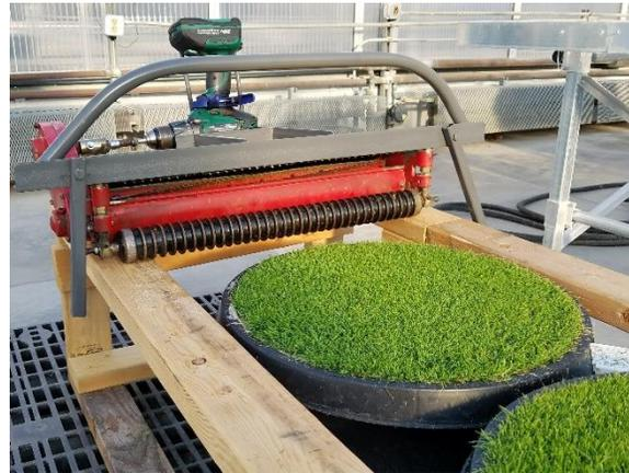
Mowing turf in the greenhouse is always a challenge. Craig built this great mower to help us simulate a golf fairway in a growth chamber. [Watch](#)
