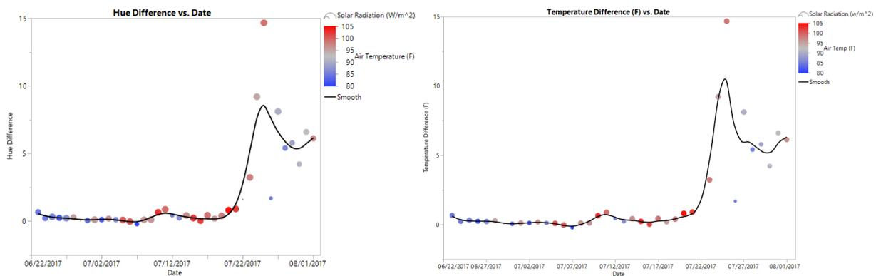
These graphs show the difference in the color/hue (left) and surface temperature (right) of well-watered and never-watered turf. The surface temperatures spike above the temperature of the well-water turf only after visible drought was detected on July 22.
