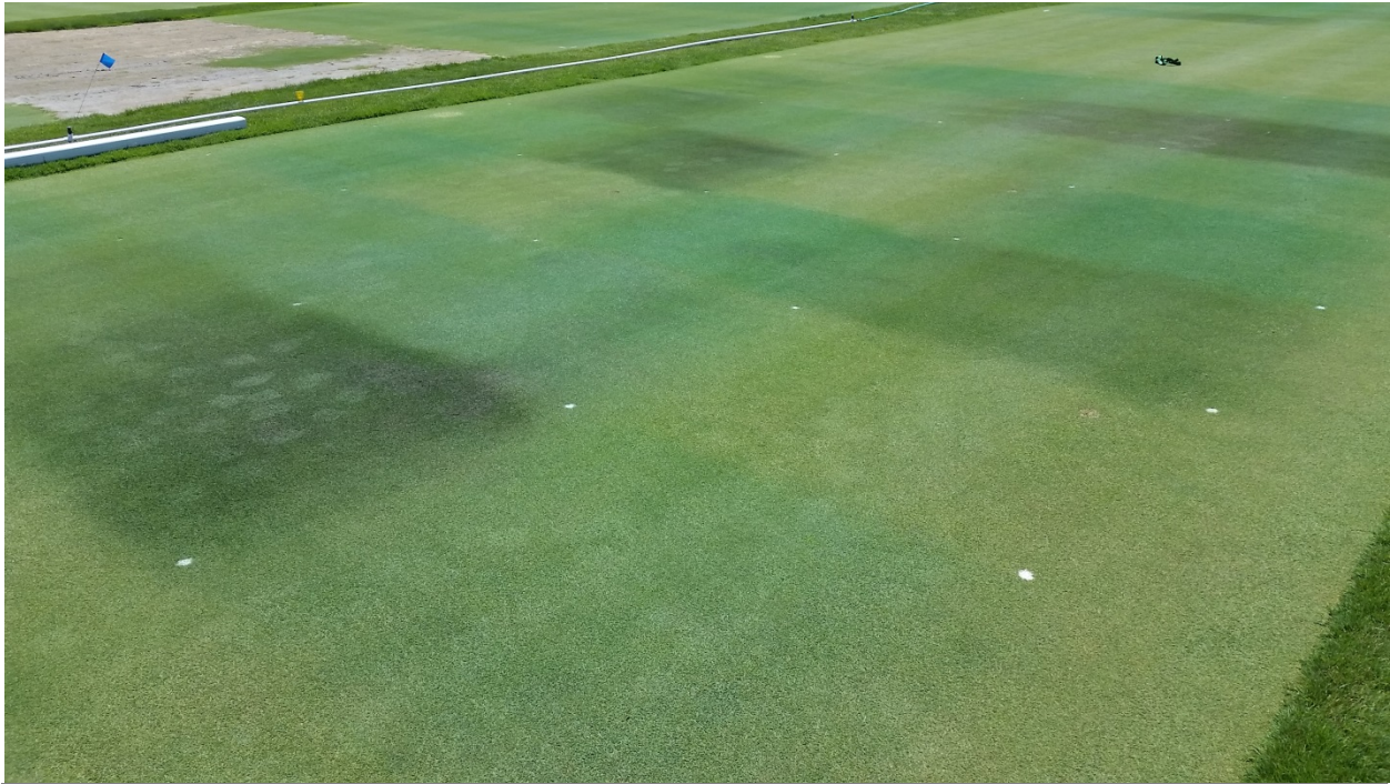
Figure 2. Turf colorants are being evaluated under three different growing environments on the Hadwick green. These plots are kept at less than 5% soil moisture with a new rainout shelter. Some colorants dry down faster than others. See more at Field Day!
